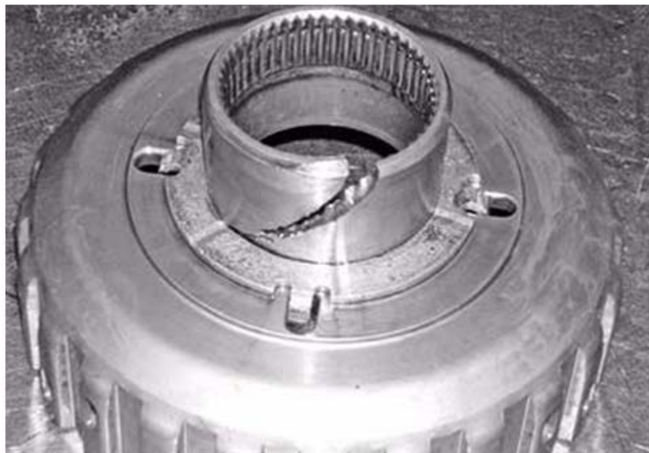
Broken C-2 clutch hub Allison 1K/2K
